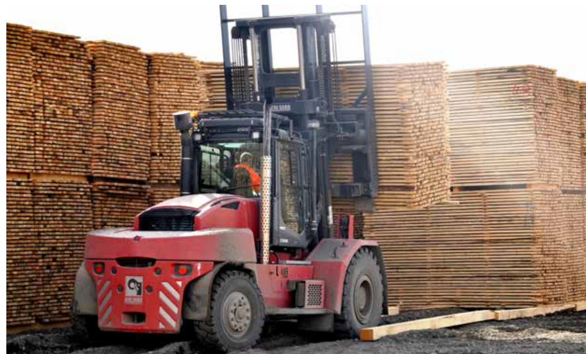
Designed specifically for the lumber industry: An optional reversible cooling fan helps clear the cooler from harmful dust. An optional rotatable driver's seat lets the driver go 'forward in reverse' with unobstructed view even when fully loaded.
